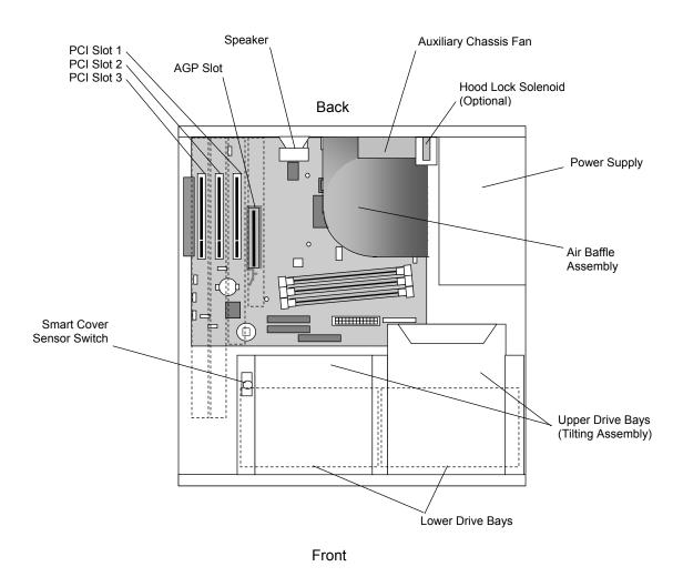
Figure 2–5. Desktop Chassis Layout, Top View
